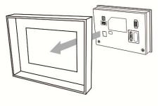
Step 3: Tighten the screws with the torque less than case DOP-107BV torque: 6.17 lb-inch (0.7 N-M)
